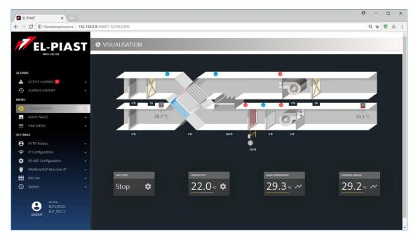
The ELP11R32 controller has Ethernet interface, so in order to connect the controller wirelessly to a local wireless network (Wi-Fi), you need to apply additional router - as an access point to set up a local area network WIFI, then connect the ELP11R32 controller to the router. The network settings of the router and the ELP11R32 controller must comply. ELP11R32 ports have to be redirected to an external address of the router.
