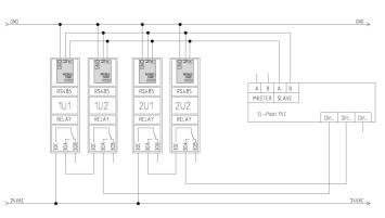
Configuration drive LG IC5 control RS485:
