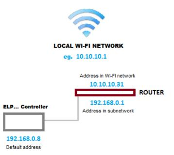
Router with port redirection: 80. From the ELP11R32 controller: 192.168.0.8:80 to sample external address of the router: 10.10.10.31. As a result we see ELP11R32 controller in local WIFI network.
