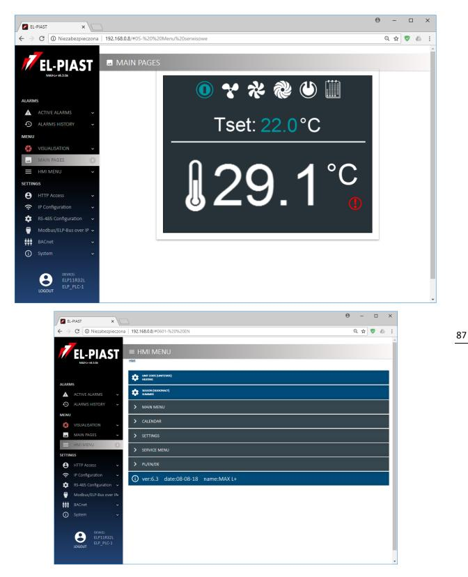
WARNING!!! The default ETH card firmware allows to use the "MAIN PAGE" text menu and the HMI Compact and HMI Advanced room menu menus "HMI MENU". The "VISUALIZATION" visualization screen on the controller's website is available only as a dedicated application for the universal application "MAX L v6.3 + 2018 08 08" or as an individual, additionally payable, with visualization acc. customer guidelines dedicated to the layout with a custom application.
