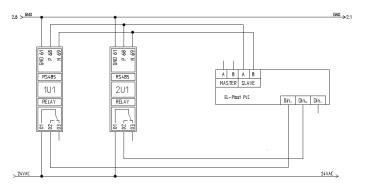
Example for system with double supply, double exhaust
