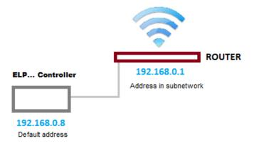
Router with port redirection: 80. From the ELP11R32 controller: 192.168.0.8:80 to sample external address of the router: 192.168.0.1. As a result we see ELP11R32 controller in local WIFI network.
