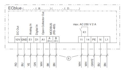
EC Blue Fan Controller Configuration - Service Menu/Fans/EC Blue Address
