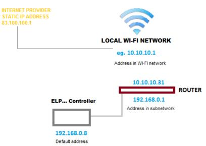
Port redirection on main Router from WIFI Router of ELP11R32 Controller: port:80 from IP:10.10.10.31 to outside IP port: 80 IP: 83.100.100.1
