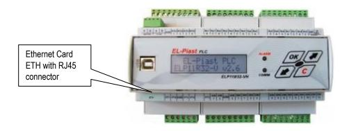
To connect from a local computer connected directly with a cable to Ethernet card ETH of the ELP11R32 controller you have to:
