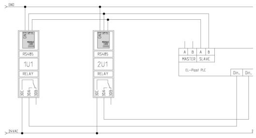
Configuration drive LG IC5 control RS485:
