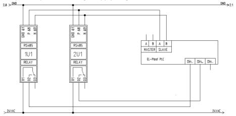
In addition, the DANFOS FC101 inputs must be shorted with numbers 12 and 27
