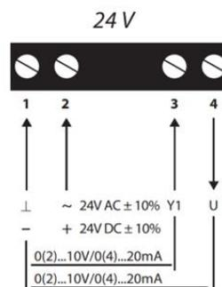
Fig. 3. Connection diagram for the 3D valve actuator
