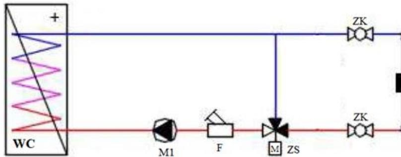
Fig. 1. Hydraulic diagram for connecting the Mixing node RSU.
