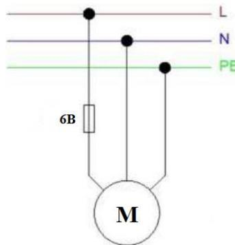
Fig. 2. Connection diagram for the circulator pump
